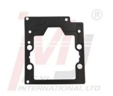
The Danfoss Series 90 100cc End Cap Gasket (Part No. 8200212) is manufactured to meet the sealing requirements of high-pressure hydraulic pump applications. Constructed from rubber-coated metal, it provides excellent sealing integrity, resistance to pressure fluctuation, and long-term durability under demanding operating conditions.
